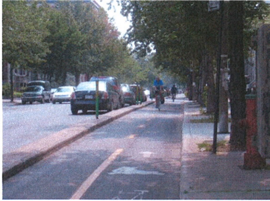
A side path in Montreal. Side paths must be separated from the adjacent roadway.
