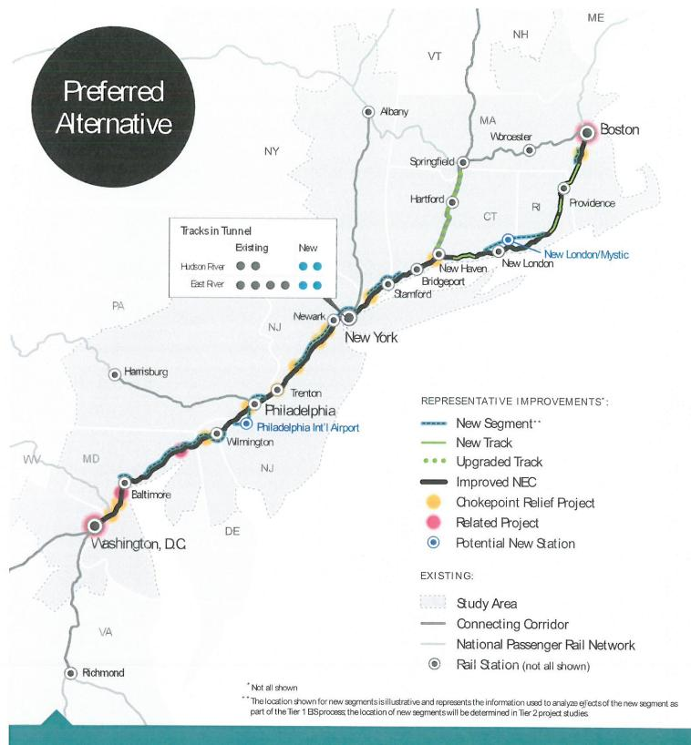
The Preferred Alternative includes improvements to bring the NEC to a state of good repair and relieve chokepoints that cause delay. It adds new track to grow the NEC to four tracks at most locations, with more tracks in areas with the greatest demand. In addition, the Preferred Alternative integrates direct service on the Hartford/Spring ald Line into the NEC, with upgraded track and electrication.
