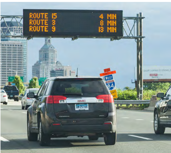
Figure 03.5 – Variable Messaging Sign
