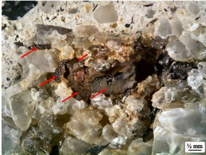
Pyrrhotite Inclusion in Coarse Aggregate (photo courtesy of Nick Scaglione)
