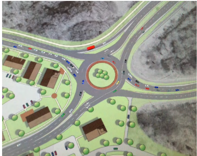
Screenshot image of the VISSIM traffic model that was developed for the preferred roundabout concept at the intersection of Route 6 and Route 66 in Columbia (Lighthouse Corners).
