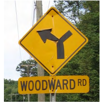
Intersection warning sign with supplemental road name plaque in Route 6 corridor, Columbia.
