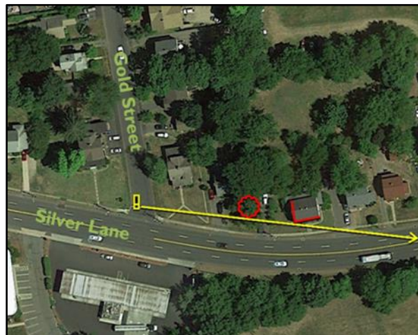
Limited Intersection Sight Distance at Gold Street
