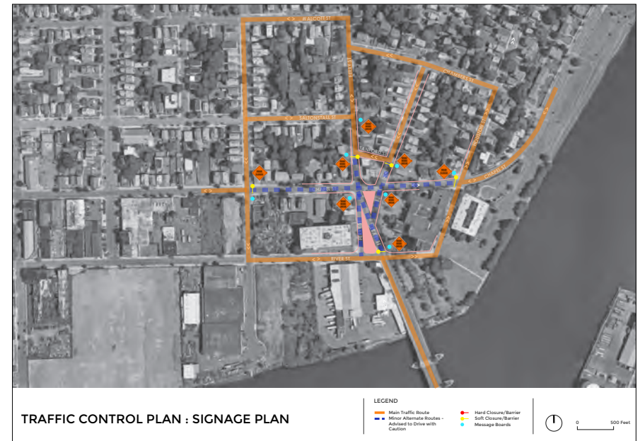
A simple traffic control plan submitted to the City of New Haven in advance of the implementation of a intersection-scale Quick-Build project. Photo: Street Plans
