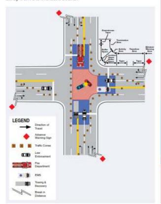
Four-Way Intersection: This is an intersection where one quadrant is blocked. It is preferred that motorists approaching the incident be restricted on which movements they can make. A flagger should be stationed within the intersection and spotters should be positioned within the advance warning and termination areas. In this example, motorists approaching from upstream are diverted around the incident scene.
