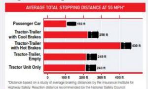
+ The overall stopping distances are doubled for wet roads and multiplied by 10 for snow and icy conditions. ESTABLISHING TTC
