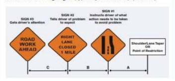
Shoulder Closure: Although a travel lane is not directly impacted/blocked, if response activities are expected to last more than a few minutes a TIMA should be established to ensure on-scene safety, including provisions for lateral buffer space. If additional lateral space is required for response or recovery activities outside of the shoulder area, the adjacent lane should be closed.
