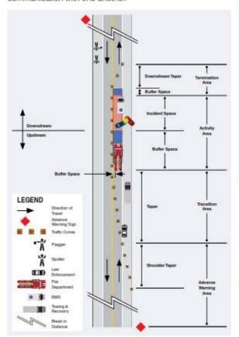
Curved Roadway: Additional advance warning is required to advise approaching motorists of the incident scene due to reduced sight distances. When possible, it is recommended that advance warning area, transition area and buffer space start upstream of the curve. Similar practices should be followed for incidents on or near hills.
