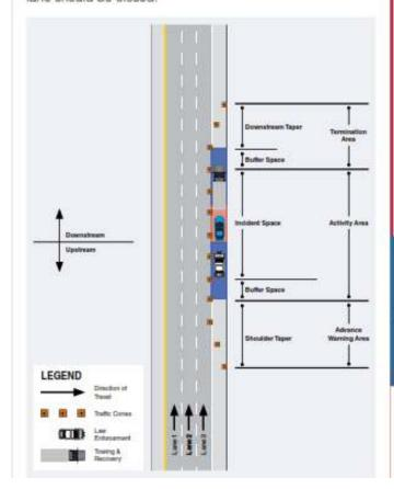
**Divided Roadway:** When establishing traffic control for incidents on this type of roadway, it is important to consider motorists' sight distance due to roadway geometry, including hills and crests.
