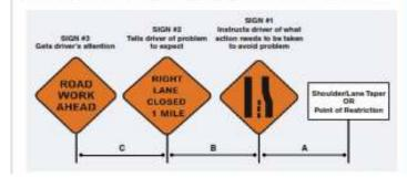
Placement of signs and devices must provide adequate guidance to motorists entering and traveling through the TIMA.
