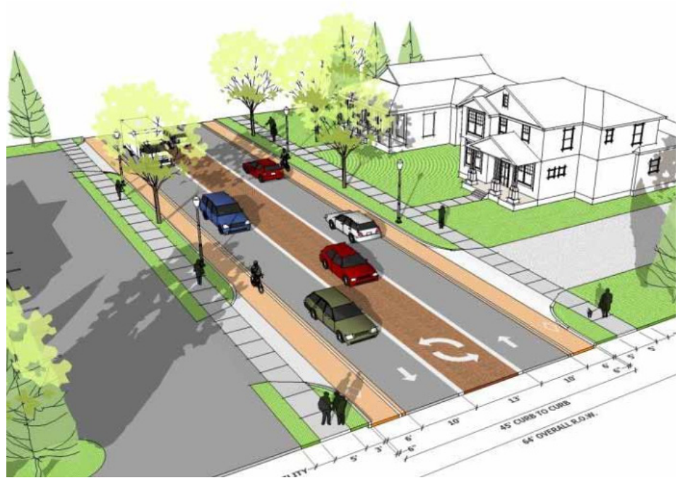
Proposed three-lane roadway section under road diet scenario
