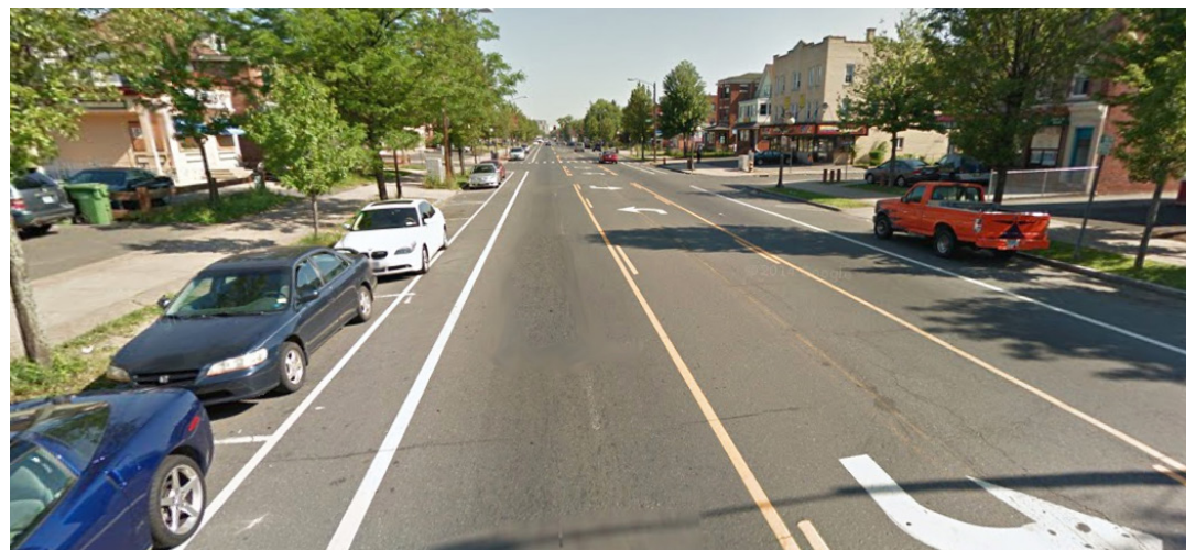
Franklin Avenue road diet with two-way left turn lane, bike lane and on-street parking.
