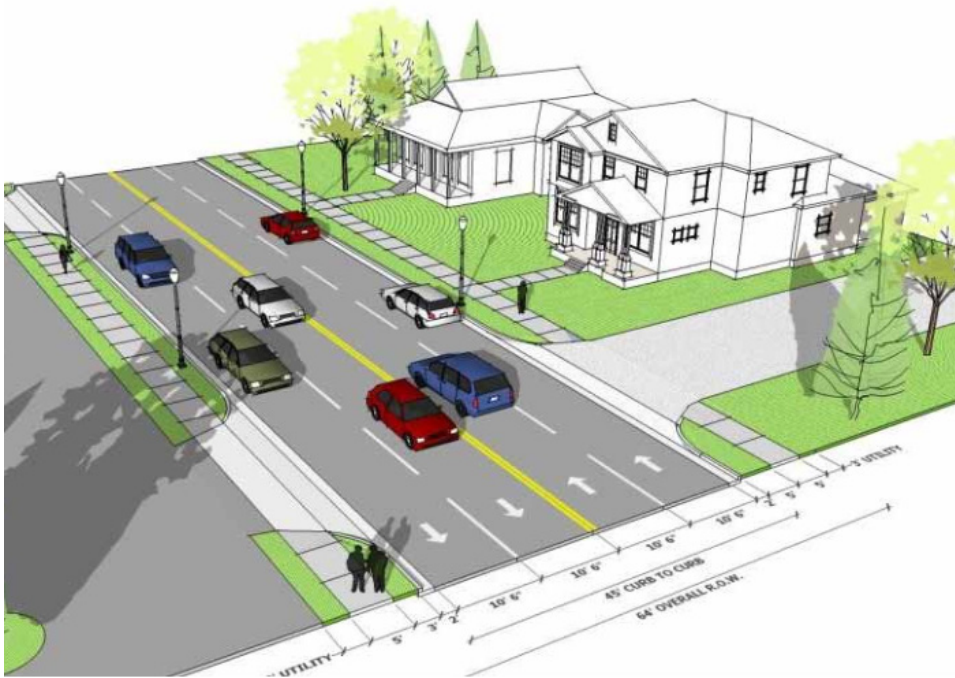
Typical section of a four- lane roadway
