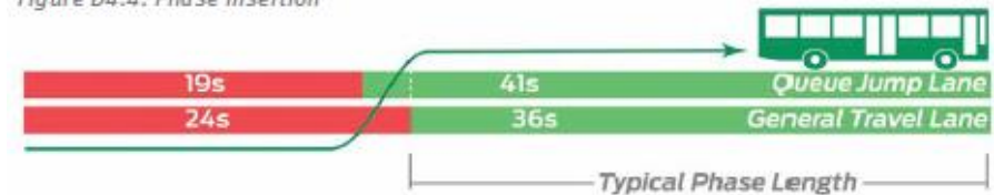
Figure D4.4: Phase Insertion
