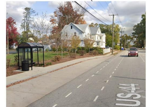
Dashed bicycle lane adjacent to bus pull out and shelter at Larrabee St
