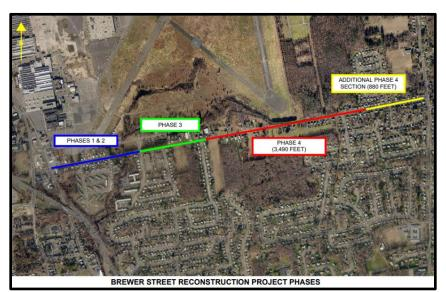
The Town originally proposed to reconstruct 3,490 linear feet of roadway on Brewer Street, terminating at #349 Brewer Street. The original proposed project also included new drainage, sidewalks, ADA compliant ramps, and 4-foot-wide bicycle lane shoulders.
