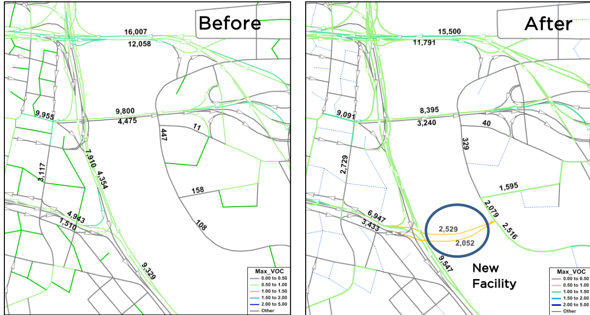
Figure 37: Comparison of AM Peak Traffic Assignment (Before / After New Facility)
