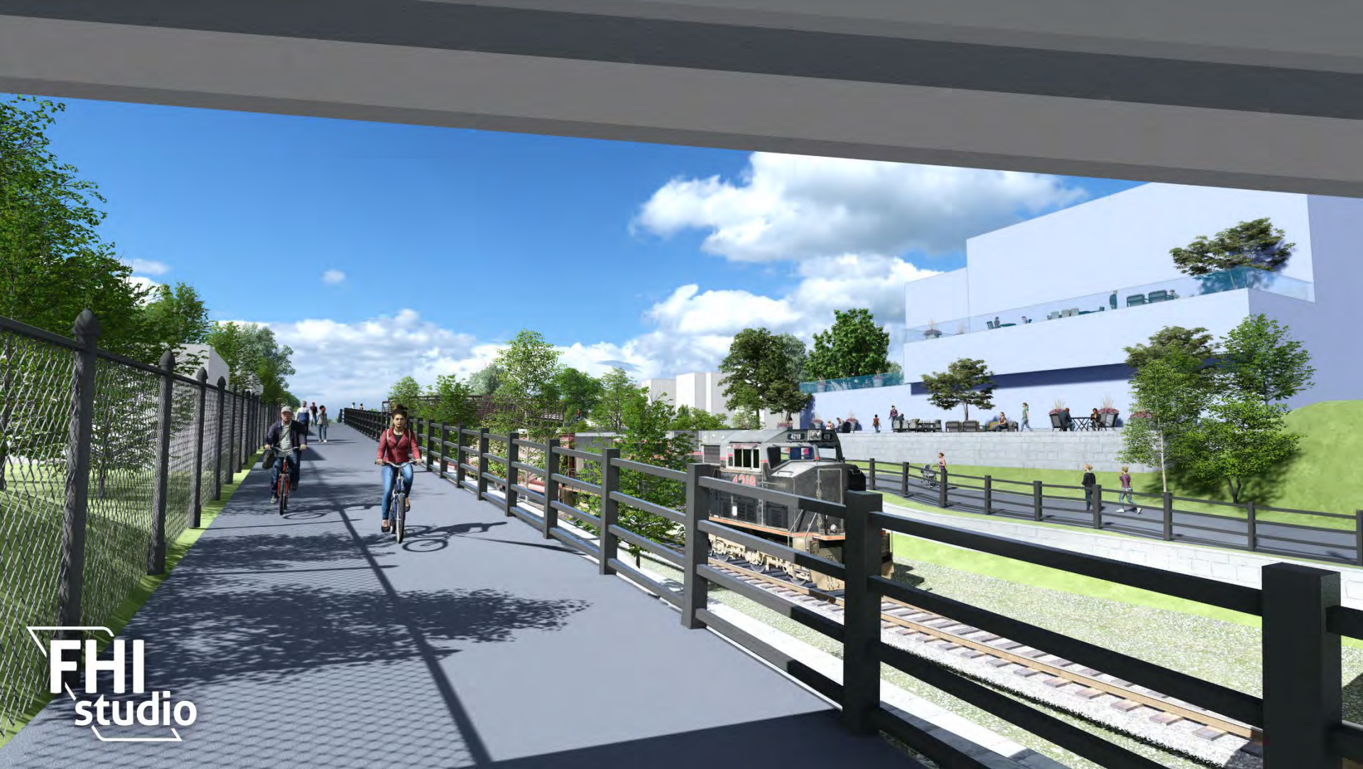
3D rendering of mainline of the Preferred Alignment on the south side of the railroad. Note the fencing proposed between the trail and railroad
