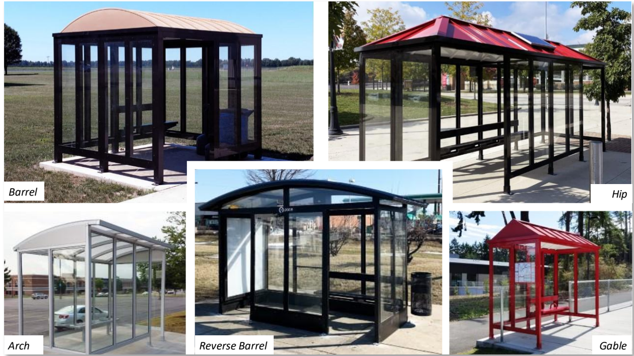
Figure 18: The palette of bus shelter roof styles selectable through the Bus Stop Enhancement Program
