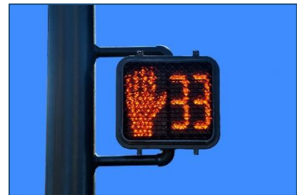
Figure 7: A crosswalk countdown signal showing the time left in a pedestrian crossing phase.
